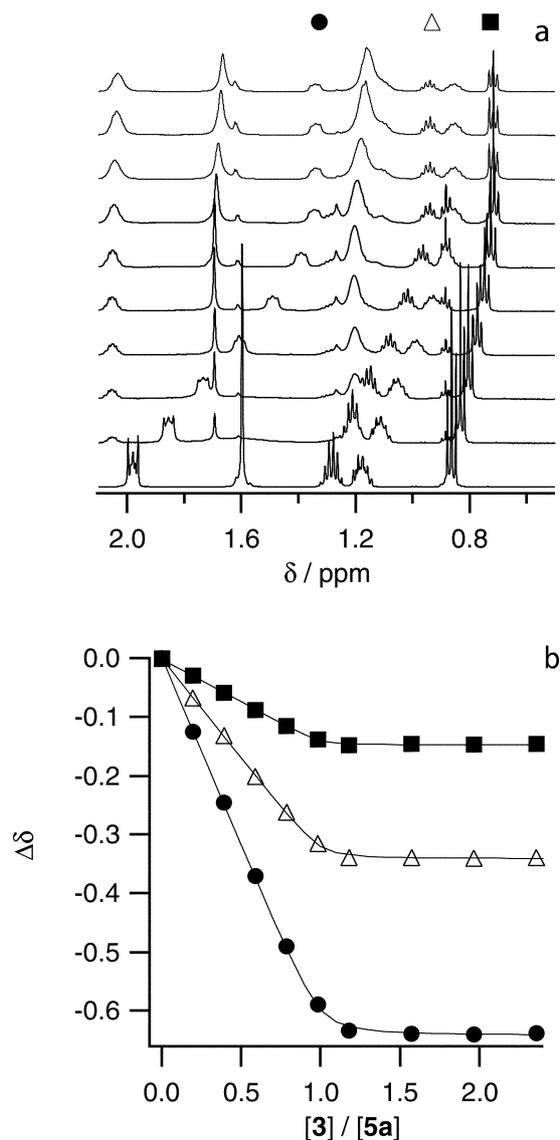
**Fig. 8** The  $^1\text{H}$  NMR titration of **5a** upon addition of **3** in  $\text{CDCl}_3$  at 298 K.  $[\text{5a}] = 1.0 \times 10^{-2} \text{ mol dm}^{-3}$ ,  $[\text{3}] = 0-2.4 \times 10^{-2} \text{ mol dm}^{-3}$  (from the bottom to the top). Methyl and methylene (C1 and C2) protons are represented by closed circles, open triangles, and closed squares, respectively.
