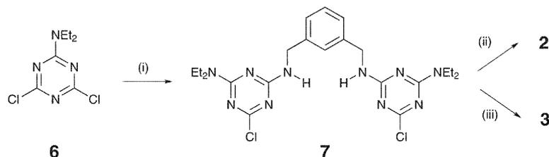
Fig. 1 Synthesis of **2** and **3**. (i) *m*-Xylylenediamine,  $\text{K}_2\text{CO}_3$ , 1,4-dioxane, rt, 84%; (ii) 1,12-diaminododecane,  $\text{K}_2\text{CO}_3$ , 1,4-dioxane, reflux, 50%; (iii),  $\text{K}_2\text{CO}_3$ , 1,4-dioxane, reflux, 43%.
