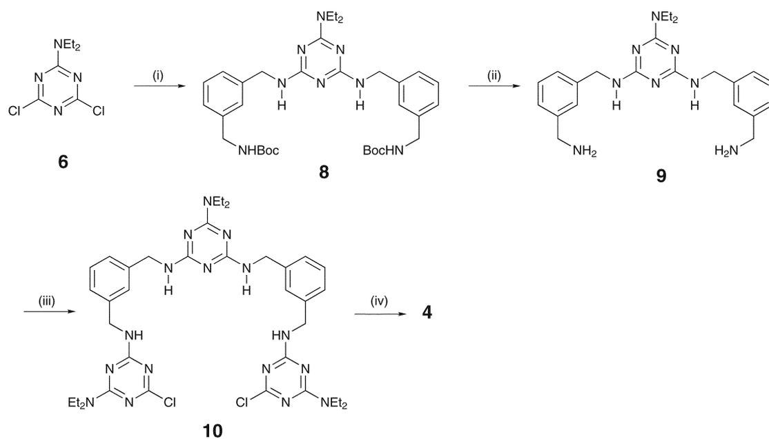
**Fig. 2** Synthesis of **4**. (i) 3-*tert*-Butoxycarbonylaminoethylbenzylamine,  $\text{K}_2\text{CO}_3$ , 1,4-dioxane, reflux, 98%; (ii)  $\text{TFA-H}_2\text{O}$ , rt, 85%; (iii) 2,6-dichloro-4-diethylamino-1,3,5-*s*-triazine,  $\text{K}_2\text{CO}_3$ , 1,4-dioxane, rt, 75%; (iv) *m*-xylylenediamine,  $\text{K}_2\text{CO}_3$ , 1,4-dioxane, reflux, 15%.
