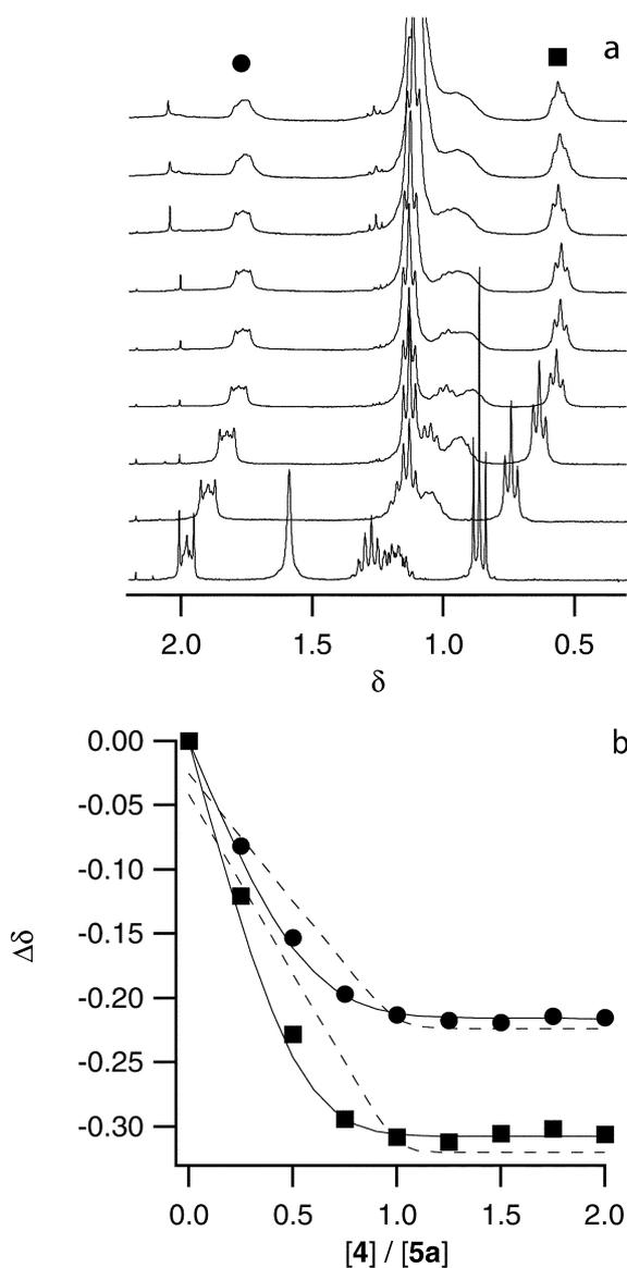
**Fig. 7** The  $^1\text{H}$  NMR titration of **5a** upon addition of **4** in  $\text{CDCl}_3$  at 298 K.  $[\text{5a}] = 1.0 \times 10^{-2} \text{ mol dm}^{-3}$ ,  $[\text{4}] = 0-2.0 \times 10^{-2} \text{ mol dm}^{-3}$  (from the bottom to the top). The solid and dashed lines indicate calculated binding isotherms based on host : guest = 1 : 2 and 1 : 1 models, respectively. Methyl and methylene protons of butyl groups of **5a** are represented by closed squares and circles, respectively.
