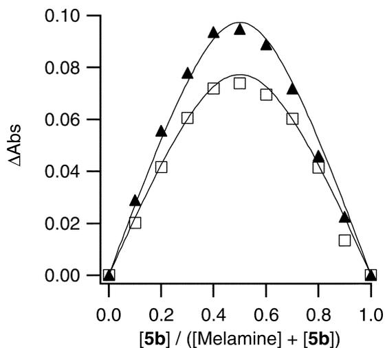
**Fig. 4** Job's plots for complexation of **5b** with **3** ( $\blacktriangle$ ) and **4** ( $\square$ ). Determined by UV-vis spectroscopy.  $[\mathbf{5b}] + [\text{melamine}] = 1.0 \times 10^{-4} \text{ mol dm}^{-3}$  in  $\text{CHCl}_3$  at 298 K.
